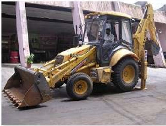
Photo 7a: Excavator cum loader
