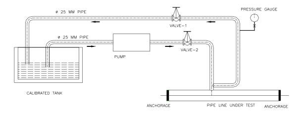
(v) **Procedure**: Pressure gauge of 150 mm diameter and pressure rating 1.5 to 2 times test pressure should be installed. The pressure gauge should be
