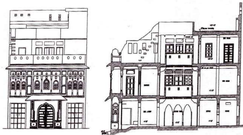
Front facade and section of a haveli
