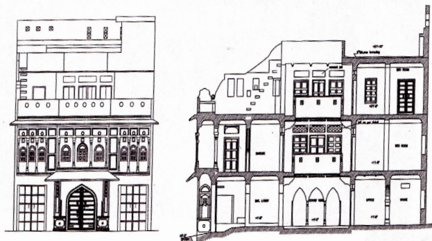
Front facade and section of a haveli
