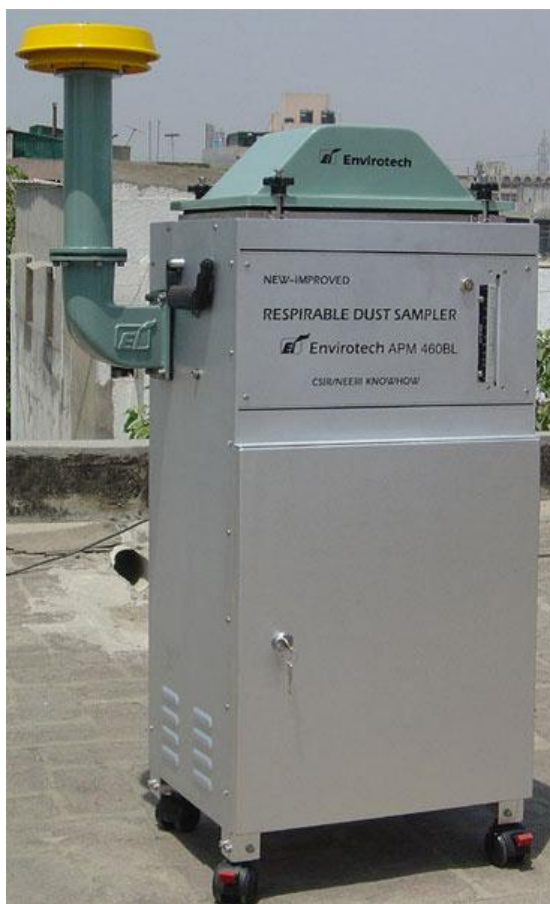
Figure: 3.9 Respirable Dust Sampler used for monitoring of Ambient Air quality
